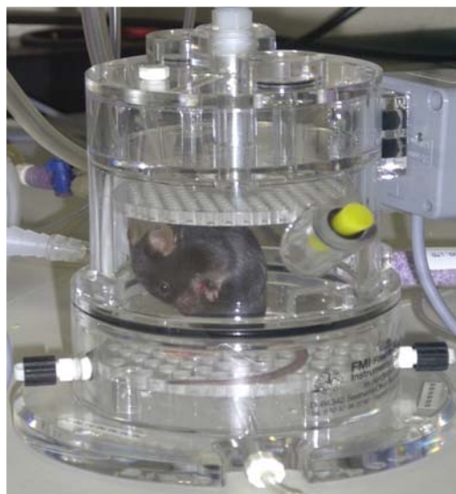
Figure 5: System used at GMC to assess breathing patterns.
