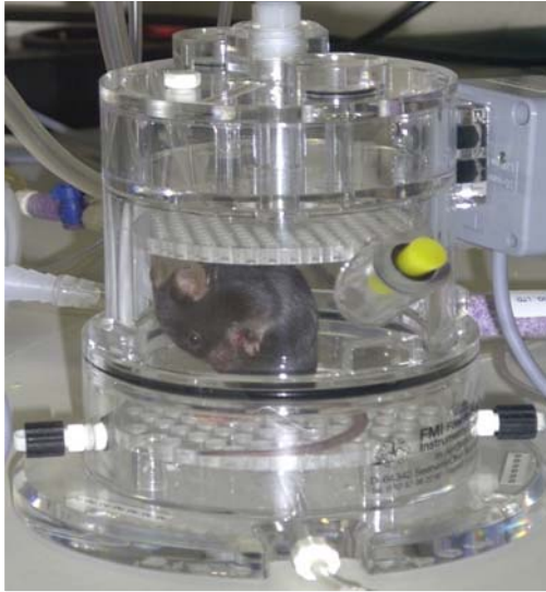
Figure 3: System used at GMC to assess breathing patterns.
