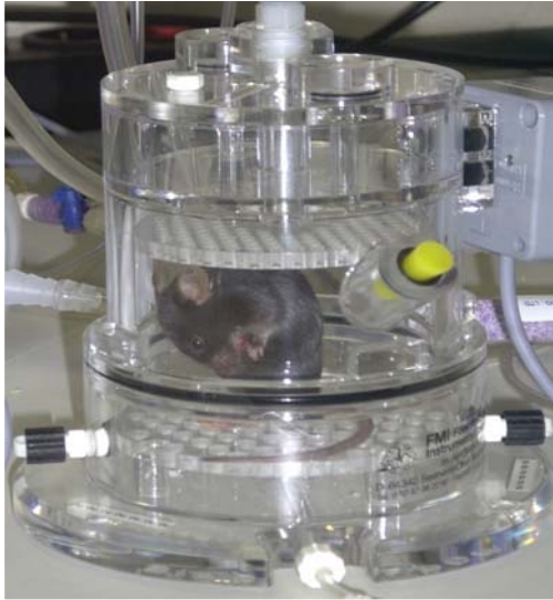
Figure 6: System used at GMC to assess breathing patterns.
