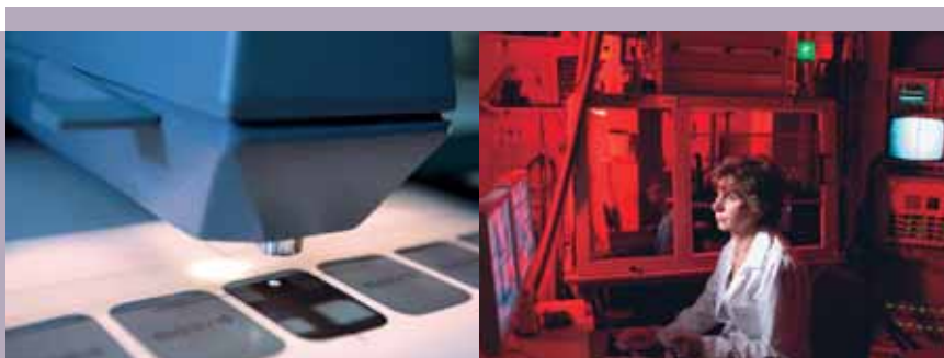
When developed dosimeter film darkens in proportion to the amount of radiation energy received. Due to the differing amounts of filtration information can be gained on the energy of radiation causing the dose.
