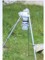
In-situ gamma spectrometry for measurement of natural radionuclides in soil
